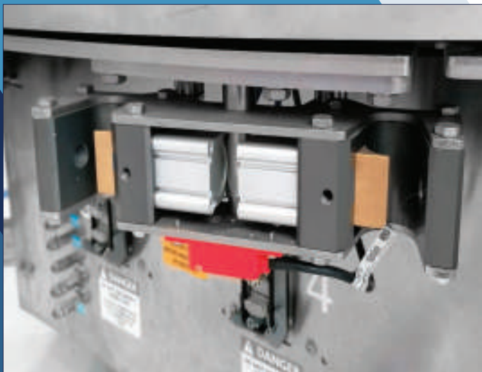
PNEUMATIC connection of removable modules (Optional)
