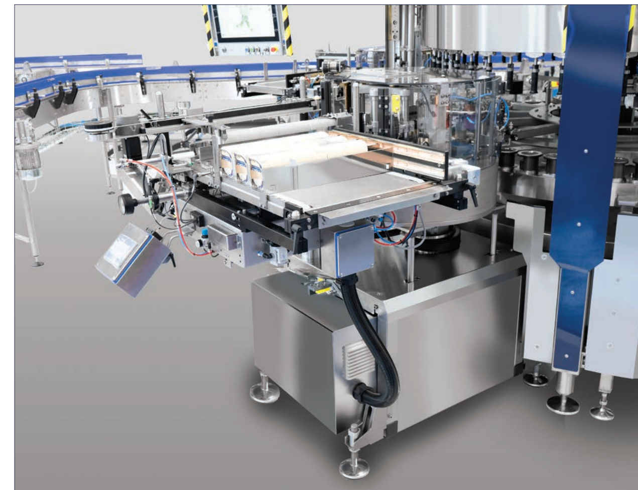
MAK-GHS station with automatic label magazine
